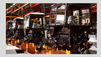
A tractor manufacturer and agricultural equipment company switched its final assembly line management to JIS and increased the number of models produced from 8 to 16. This marked a 100% increase in models with no increase in inventory or production space.
